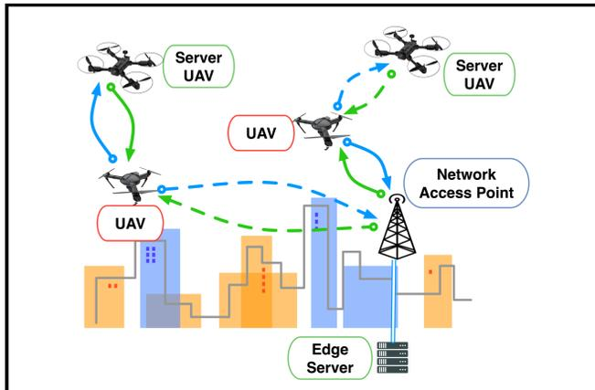
**UAVs have limited energy/computing power due to weight constraints**
