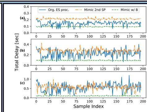
Temporal series of capture-to-output per-frame delay for (a) low, (b) medium, and (c) high external traffic load
